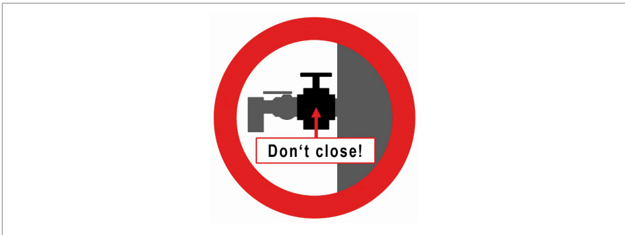
Figure 52: Slide valve warning sign
